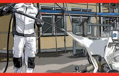
Inner tube : high temperature black nitrile rubber Outer cover : abrasion resistant neoprene rubber blue or black Application : for high pressure cleaning at 400 bar Temperature : -30°C to +120°C, intermittent 150°C WP 400 bars - BP 1200 bars
