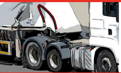
Inner tube : black EPDM rubber Outer cover : wrapped black EPDM rubber Reinforcement : metal plies Application : to convey hot compressed air exempt of oil Temperature : -40°C to +208°C WP 20 bars - BP 175 bars
